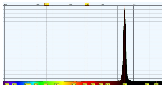
FIG. 10. Measured emission spectrum of potassium. The measured spectrum displays a dominant emission line at 773 nm, in good agreement with the expected position at 770 nm. The horizontal axis represents wavelength (nm), and the vertical axis shows intensity in arbitrary units.
