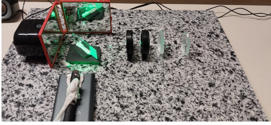
FIG. 3. An image of the final experimental setup. Laser beam, loudspeaker, microscope lamella (as a beam splitter), mirrors and lenses are shown in the figure.
